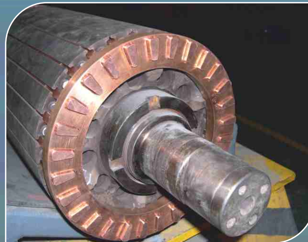
ROTOR WITH MIPALLOY 3ZR (Cr Zr Cu) SHORT CIRCUIT RINGS
