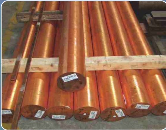
Ø200 MIPALLOY 3ZR (Cr Zr Cu) BILLETS
