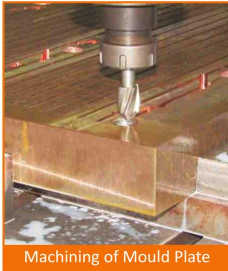
Machining of Mould Plate
