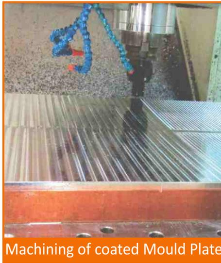
Machining of coated Mould Plate
